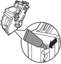
3 Apply some grease around the shaft in the bottom of the brew group.
