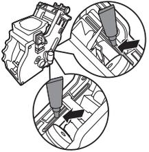
4 Apply some grease to the rails on both sides (see figure).
