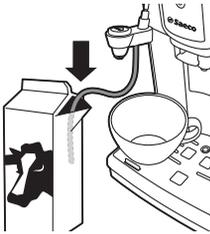
3 Insert the suction tube into a milk container.
