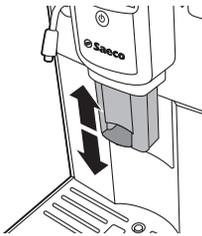
The machine can be used to dispense different coffee types in cups or glasses of different sizes. To adjust the height of the coffee dispensing spout to the size of the cup or glass, slide the spout up or down.
