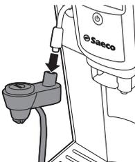
1 Remove the automatic milk frother from the hot water/steam dispensing spout.
