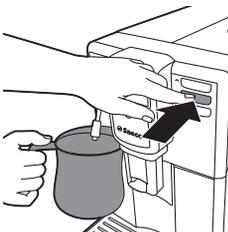
2 Place a container under the hot water/steam dispensing spout and press the HOT WATER button.
