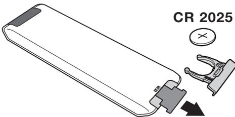
Pull out the plastic insulation sheet from the battery, this will activate the remote control. The battery supplied with the appliance does not contain mercury or nickel cadmium so as to protect the environment. Please do not discard your used batteries, but use the recycling methods available (consult your distributor).
