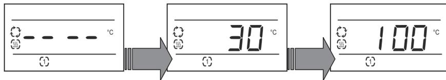
The appliance is equipped with a quick start function to heat water to 100°C in the shortest amount of time.
