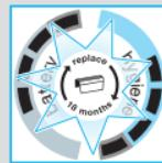
After you have replaced the Foil & Cutter cassette, use a ball-pen to push the reset button ⑯ for at least 3 seconds to reset the counter. While doing so, the replacement light blinks and goes off when the reset is complete. The manual reset can be done at any time.
