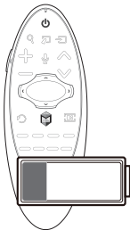
<Low battery Alarm Icon>
