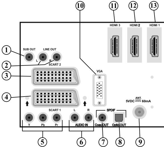
1. **Subwoofer Out** is for connecting an external, active subwoofer to the set to give a much deeper bass effect.
