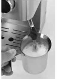
**NOTE:** To make steamed milk, the portafilter with filter insert has to be in the brewing group!
