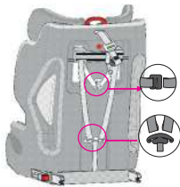
Removal of the belt lock
