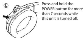
Press and hold the POWER button for more than 7 seconds while this unit is turned off.
