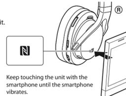
Keep touching the unit with the smartphone until the smartphone vibrates.
