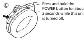
Press and hold the POWER button for about 2 seconds while this unit is turned off.
