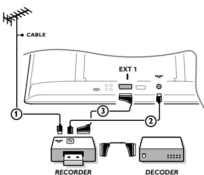
Connect the aerial cables ①, ② and, to obtain the optimum picture quality, eurocable ③ as shown.
