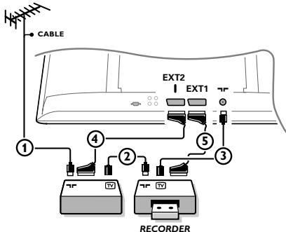
Connect the aerial cables ①, ② and ③ as shown (only if your peripheral has TV aerial in-/output). Connect your equipment with a eurocable ④ or ⑤ to one of the euroconnectors **EXT1** or **2** to obtain a better picture quality.
