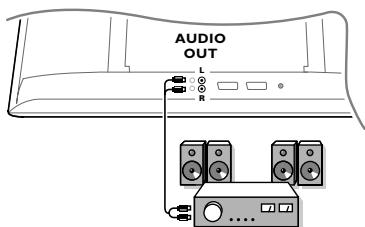
To connect to a hi-fi system, use an audio connection cable and connect the **L** and **R AUDIO** outputs on the TV set on the **AUDIO IN L** and **R** input on your hi-fi amplifier.
