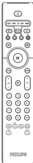
Press the **Select** key to select the required mode : **VCR**, **DVD**, **SAT**, **AMP** or **CD**. The remote control indicator lights up to display the selected mode. It switches off automatically after 60 seconds if left idle.
