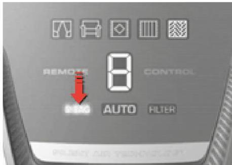
**1. Models with digital display: Change the dust bag when the s-bag® indicator is illuminated.\***
