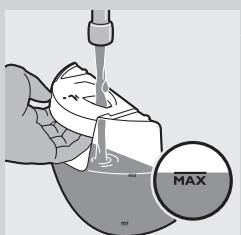
**2 Fill the water tank with tap water up to the MAX indication.**
