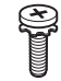
Stand Screw 5 EA, M4 x L14 (Only 55EF95**) 8 EA, M4 x L14 (Only 65EF95**) (See p. A-7, A-9)
