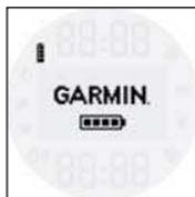
4. Charge the Forerunner completely. When the Forerunner is fully charged, the animated battery on the screen is solid (
