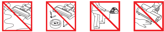
Do not pick up water or liquids. Do not pick up burning objects. Do not use above you on the stairs. Do not put hands near the brush bar when the appliance is in use.
