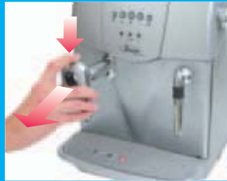
Remove the brew unit and wash it with water.
