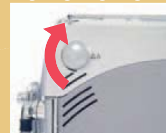
Turn the knob clockwise to terminate the circuit-loading process.
