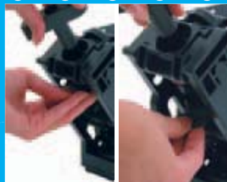
Unscrew the upper filter and wash it.
