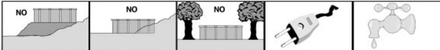
check that the site is absolutely level: correct any unevenness before assembling the pool. if the area is slanted, always take out earth from the higher part, rather than filling in lower parts.
