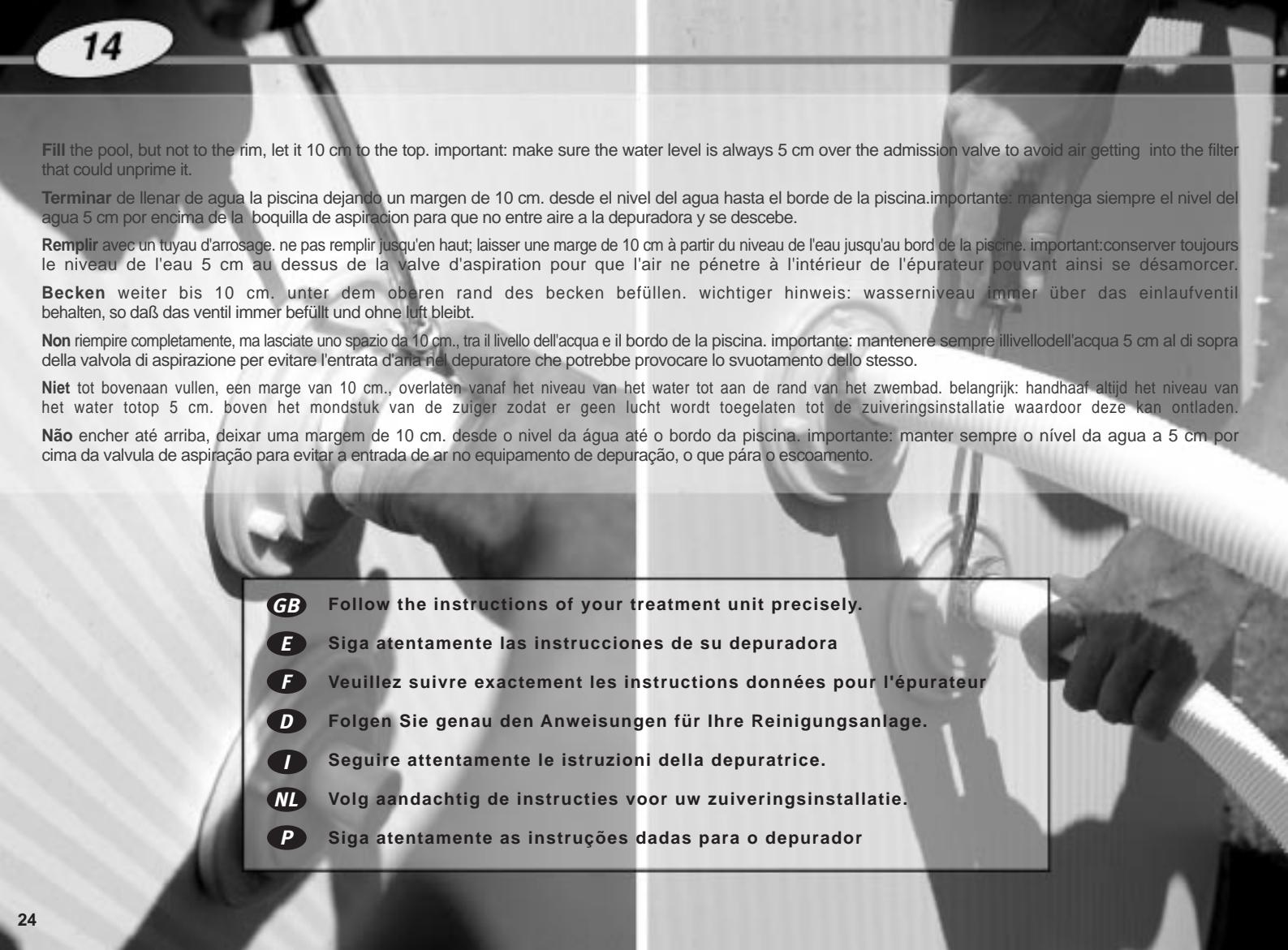
Fill the pool, but not to the rim, let it 10 cm to the top. important: make sure the water level is always 5 cm over the admission valve to avoid air getting into the filter that could unprime it.
