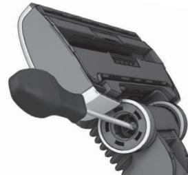
3. Unscrew the wheel axis and clean all parts.
