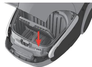
8. Replace or wash the motor filter when dirty or after every 5th s-bag. Push the filter holder down and pull it out. Exchange the filter or wash it, see step 9.
