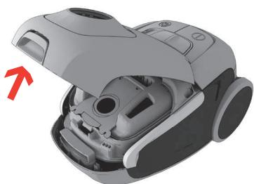
1. Open the dust compartment cover. **Check that the s-bag® is in place.**
