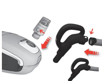
2. **Insert the hose** (to remove it, press the lock buttons and pull the hose out). Insert the hose into the hose handle until the catches click to engage (press the catches to release the hose).
