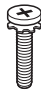
Stand Screws 4 EA, M4 x L21 (Only UB83**-ZG, UF695*-ZA) (See p. A-3)
