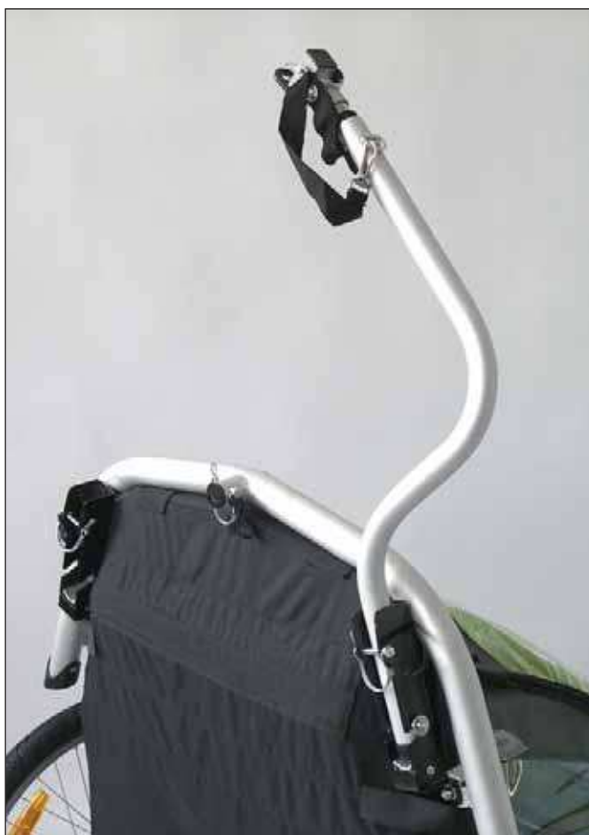
Correctly fitted hitcharm – seen from below
