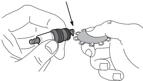
**Note:** In some areas, local law requires using resistor spark plug to suppress ignition signals. If this engine was originally equipped with resistor spark plug, use same type for replacement.
