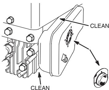
**Muffler Area & Spark Arrester**
