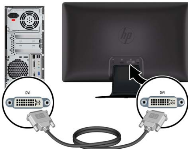
Figure 3-5 Branchement du câble DVI-D (non fourni)
