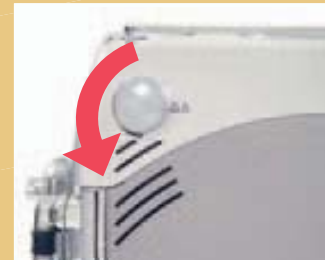
Turn the knob counterclockwise to start loading the circuit.
