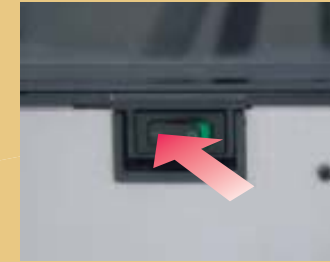
Move the ON/OFF switch to "I" to turn on the machine.
