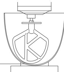
**dough hook** - this tool is set at the factory and should require no adjustment.
