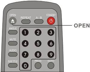
Press **OPEN** button on the remote control (or front panel) to open the disc tray. Load a disc and press **OPEN** again to close the disc tray.
