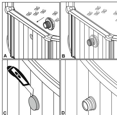
**NOTE:** Before connecting valve to the pool, fill the pool leaving 5 - 6cm of space between the position of the connection valve and water surface.
