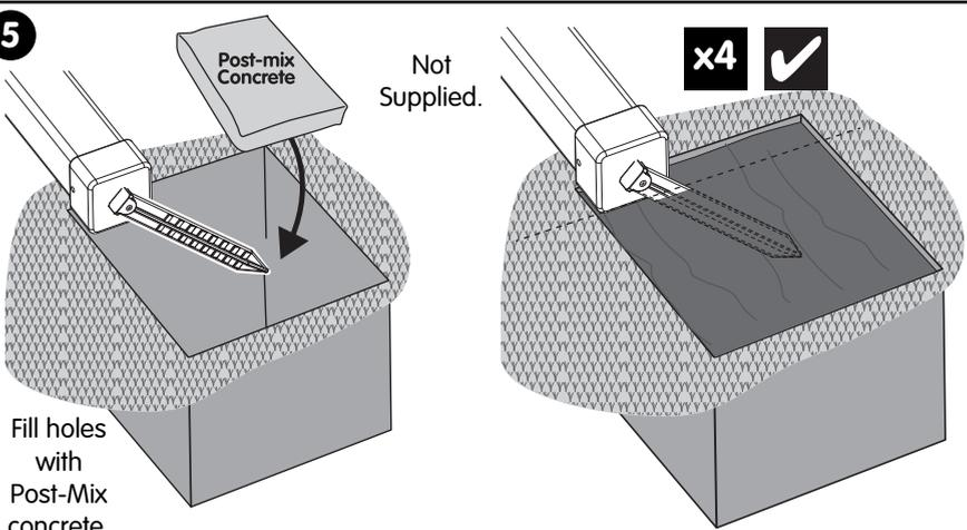
Fill holes with Post-Mix concrete.
